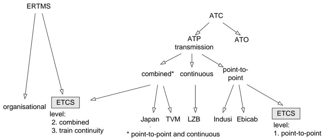
Fig. 15. ATP systems within ERTMS and ATC systems
