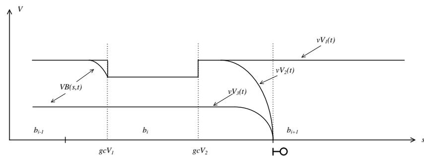
Fig. 8. Charts of safe speed as a function of displacement
