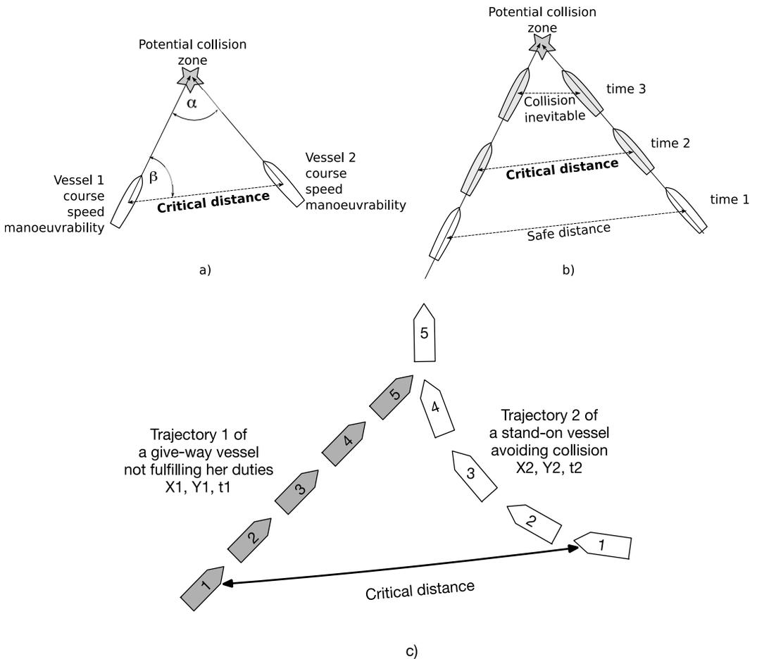
Fig. 1. A graphical representation of a concept of critical distance in ship-ship collision encounter.
