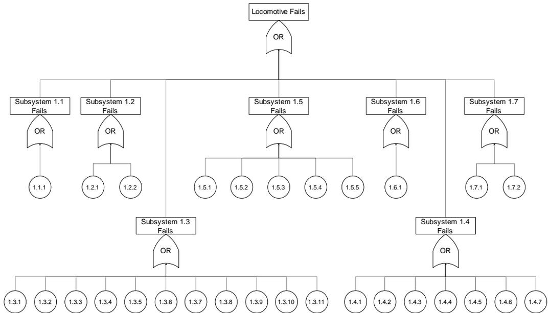
Fig. 4. 6Dg locomotive fault tree model
