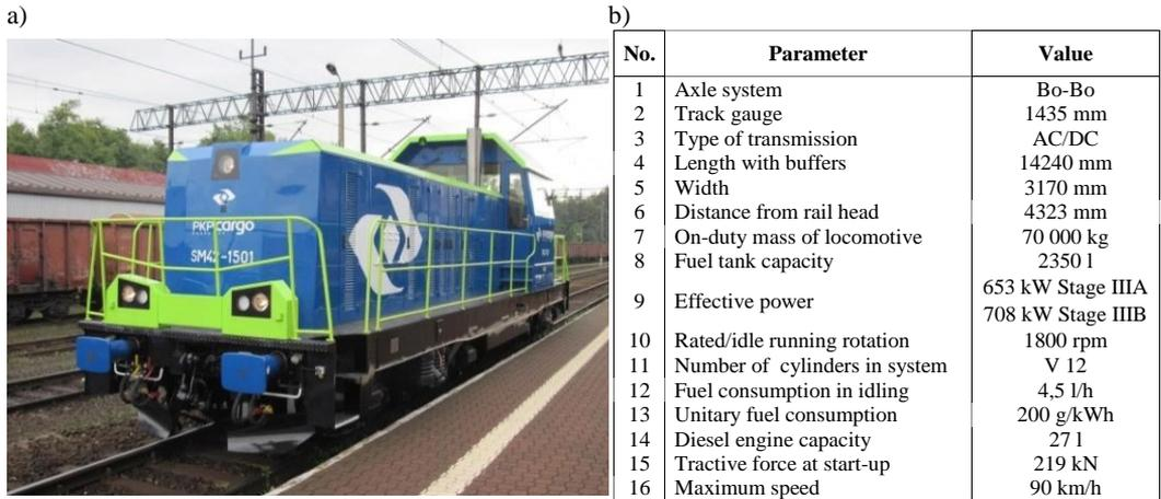
Fig.1. a) 6Dg modernised locomotive b) Selected technical parameters of 6Dg locomotive
