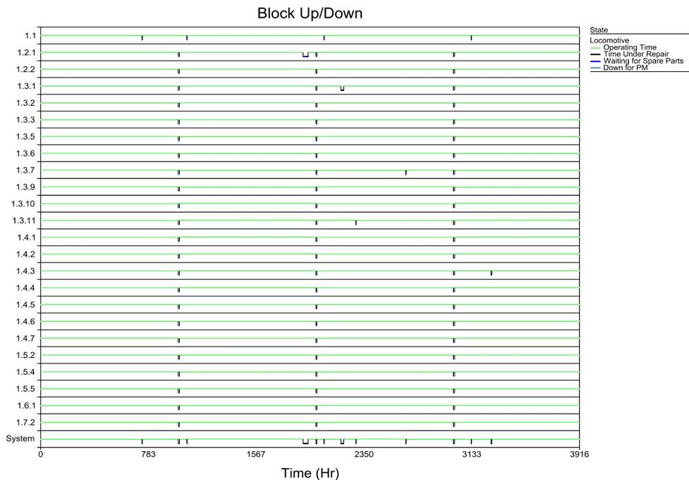
Fig. 6. State diagram (up/down) of the components and locomotive
