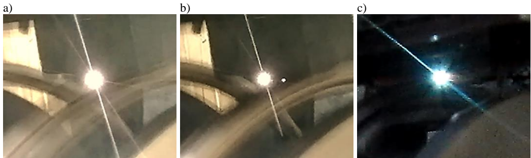
Fig. 7. Sparking in the contact zone when the omit current 500 A: a) contact strip type “A” – yellow red sparks; b) contact strip type “B” – yellow red sparks; c) copper contact strip – blue and white sparks
