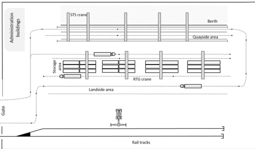
Fig 4. Marine intermodal terminal example
