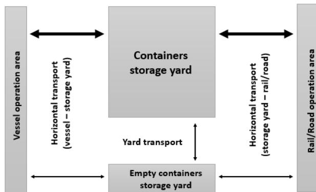
Fig. 2 Flow direction of containers in marine intermodal terminals
